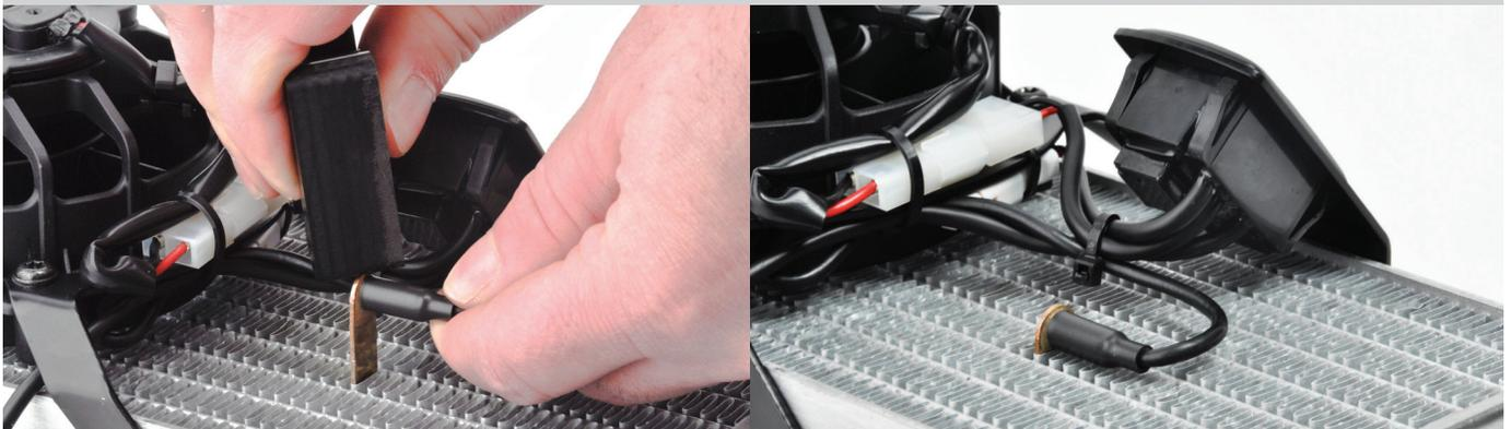
5. Carefully insert the temperature probe into fins of radiator.
