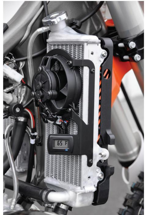
*TIP: To Compensate for the influence of ambient air passing across the sensor, apply thermal grease (included in kit) into the gap between the fins of the radiator where the sensor will be installed. It is important to place the grease only in the gap. Grease on the surface of the radiator will attract dirt and reduce function.*
